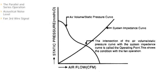
At the point, the change in slop of the air performance curve is minimized while the change in slop of the system characteristics curve is at its lowest. Note that the static efficiency (air flow times static pressure divided by power) is also optimized.
