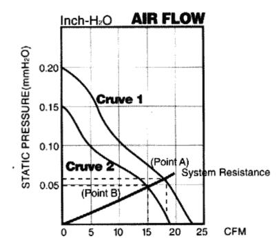
Figure #2 summarizes on one graph the change from one fan to the other. In some cases, of course, it may even be possible to move to a physically smaller fan with the same air flow, if system resistance is sufficiently reduced.
