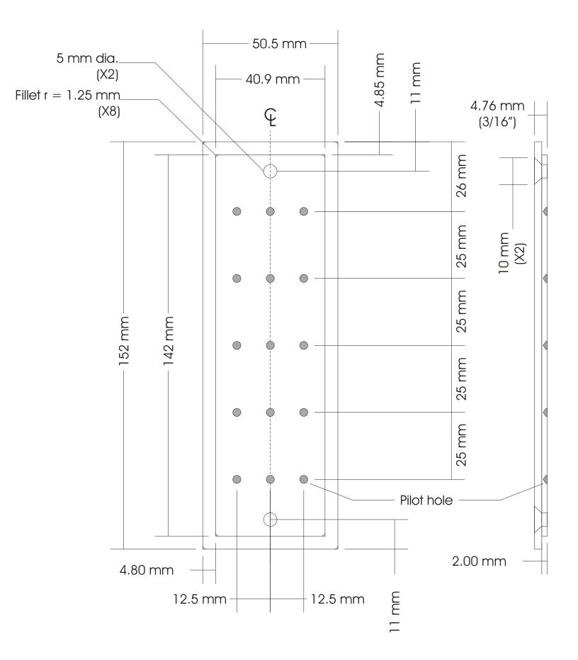
Module Faceplate Drawing SMF 03/06/2002 RW 06/26/2006 Two panels are needed per chassis assembly. Center pilot holes are the most important as they indicate where banana plugs are to be placed for power entry.
