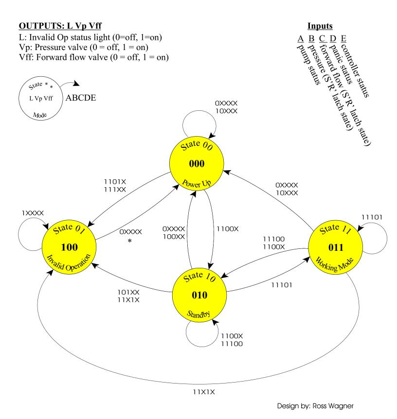
\*: From "Invalid Operation" it is possible to reset the machine to "power up" mode by simultaneously depressing both pressure and forward-flow *off* buttons.
