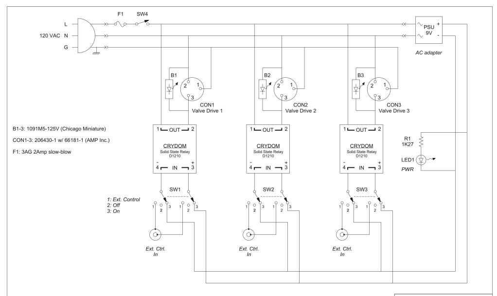
Note: The SSRs needs a minimum load of 40 mA rms to function properly. An insufficient current load may cause the SSR to conduct even if 0V is applied to the control inputs (i.e., when the relay is commanded to be off).
