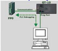
Two RS232C ports are available for connecting to the PLC and the PC. This allows you to program both the PLC and GT-10 without having to unplug any cables. It is also possible to connect a modem to
