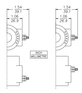
Single 8-32 Stud, Internal Ground with Diode
