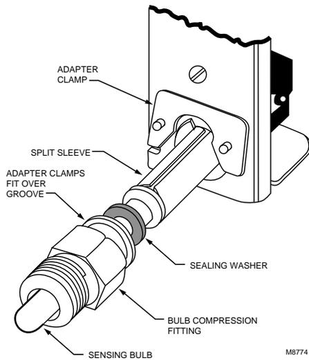
**Fig. 4—Mounting L6006C on pipe or tank.**
