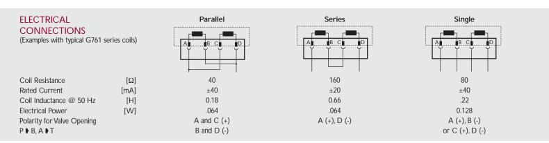
Note: Before applying electrical signals the pilot stage has to be pressurized.  $\label{eq:polyantimetric}$
