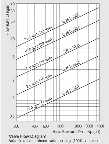
signal) as a function of the valve pressure drop.
