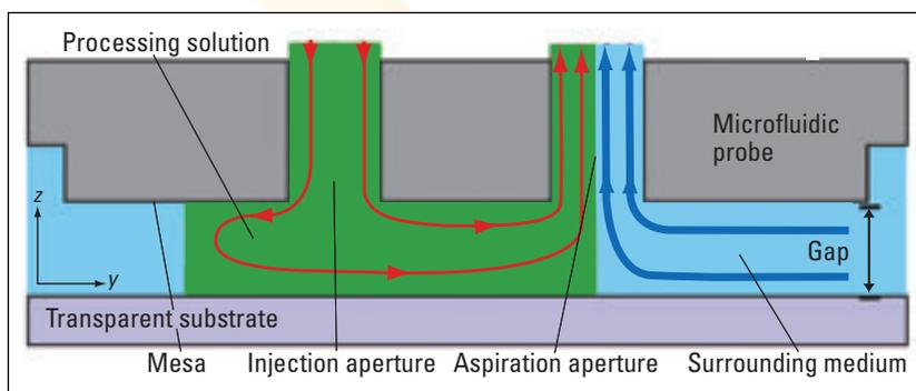
A cross-sectional schematic illustrates the mobile microfluidic probe surrounded by solution and positioned over a substrate. (Adapted with permission. Copyright 2005 Nature Publishing Group.)
